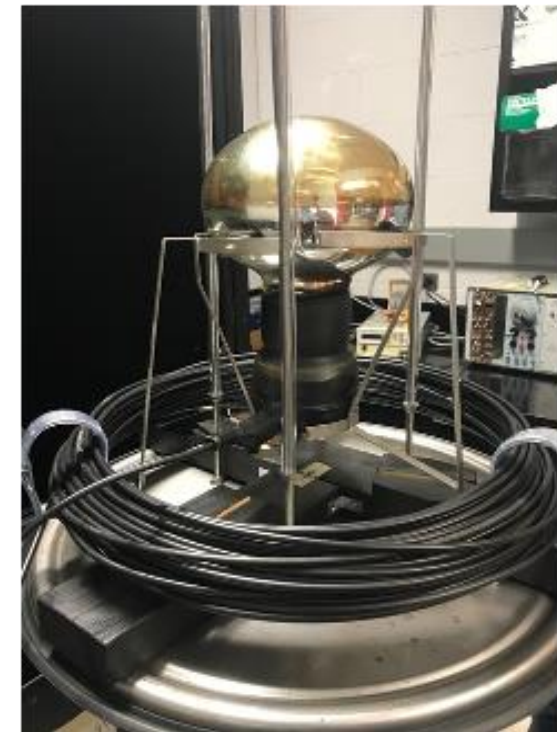
Daya Bay PMT attached to a test setup. Taken from LU PMT test facility for nEXO
