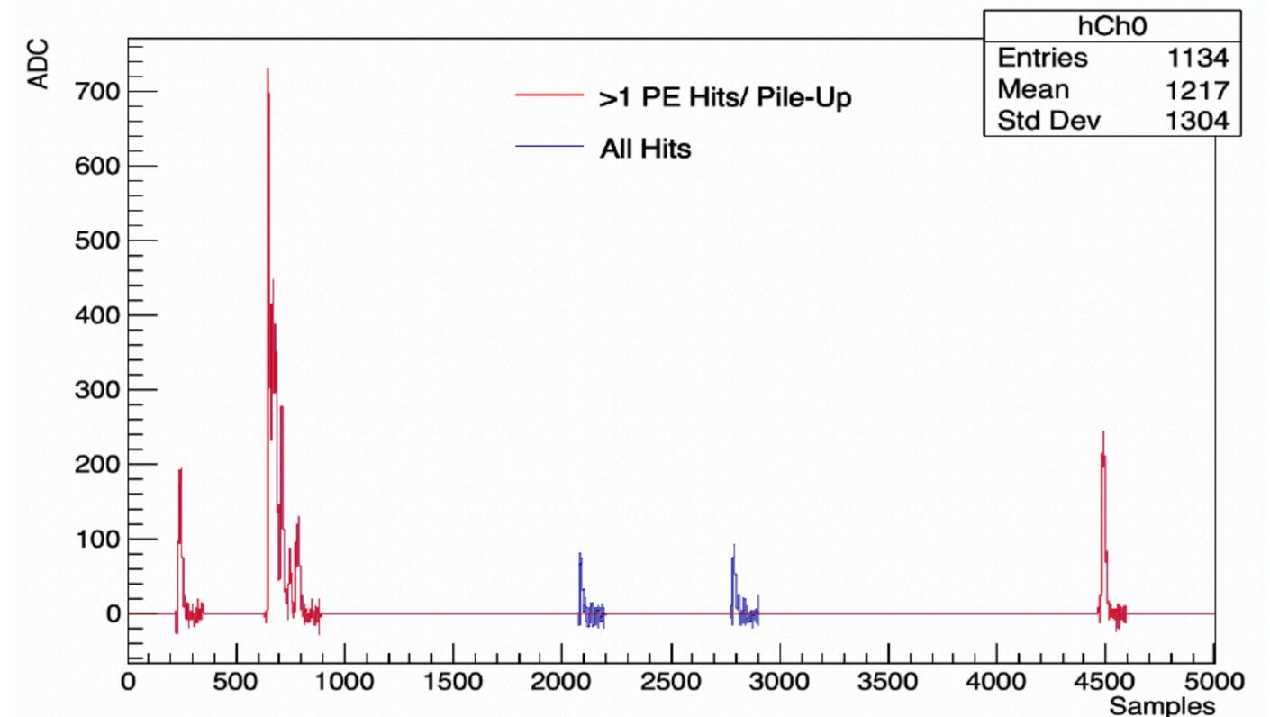
Simulated waveform of a single channel inside the inner AAr buffer (veto)
