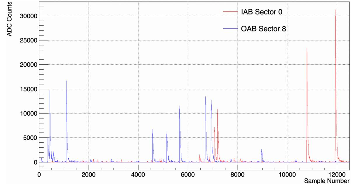
Two example summed sector WFs (one IAB, one OAB) constructed by adding together ZLE segments from individual channels of 1 ms TPC-veto coincidence window containing 1 neutron capture,  $^{39}\text{Ar}$  and background  $\gamma$ 's normalised to their expected rates
