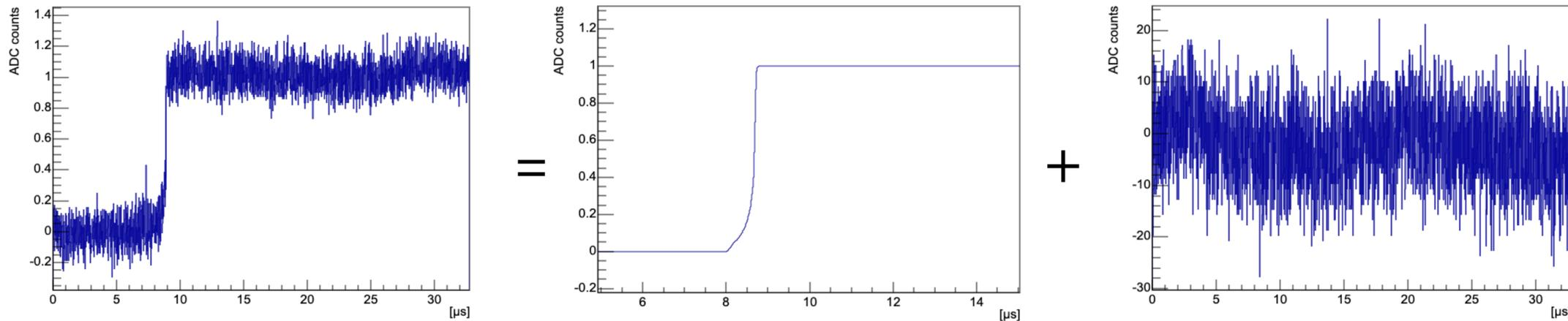
One simulated pulse was combined with 1000 different noise to make 1000 different fake pulses
