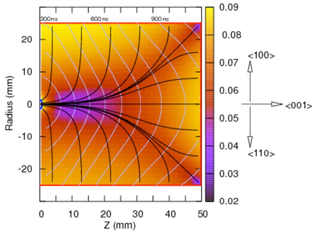
A diagram of a point-contact detector's electric field intensity (color pattern), drift trajectories (black lines), and surfaces of constant drift time (grey).
