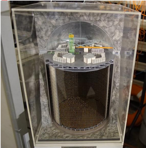
Fig: Model of Super-Kamiokande detector[2]
