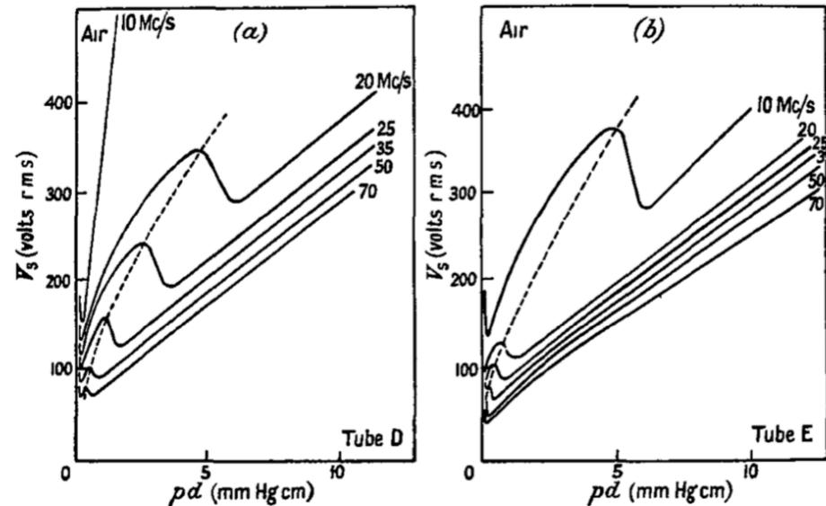
Figure 1. ( $V_s$ ,  $pd$ ) curves for air for high frequency fields.
