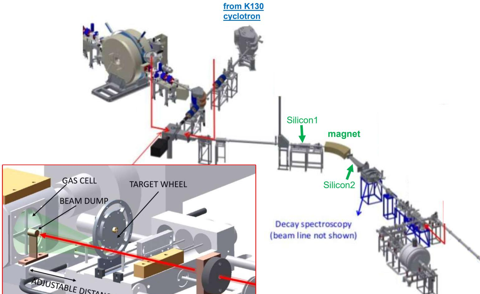
Inside target chamber (HIGISOL gas cell and platform)
