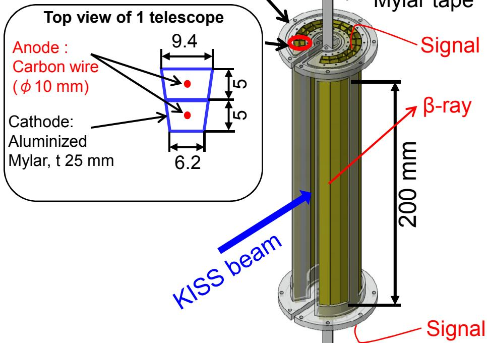
Anode wire: Carbon wire ( $\phi 10$  mm, 3 kΩ/cm)
