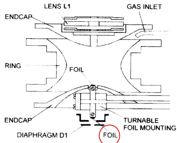
ISOLTRAP Mark 1: the collector trap
